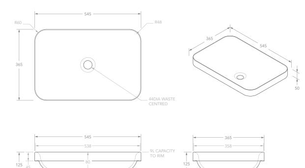
Semi-Inset Solid Surface 9L Capacity No overflow
