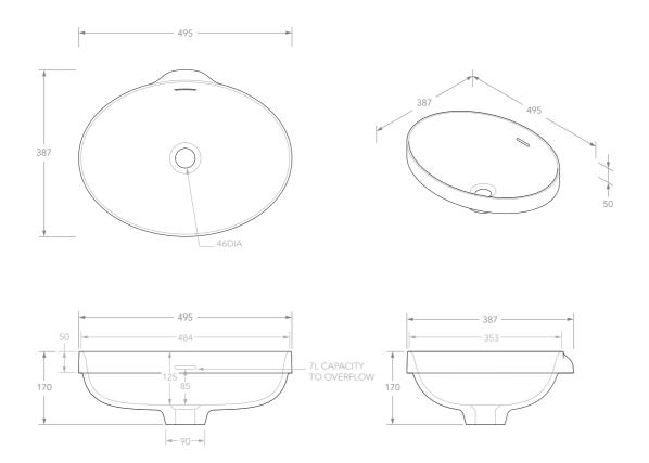
Semi-Inset Solid Surface 7L Capacity to With overflow Suits a 32mm waste with overflow overflow (ADP Universal Plug & Waste sold separately)
